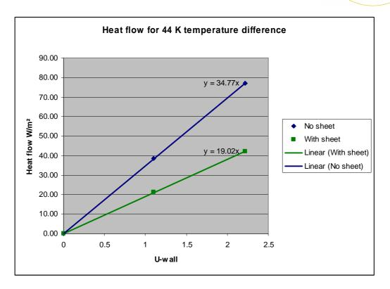
Figure 1 : Heat flow through wall for 44 K temperature difference
